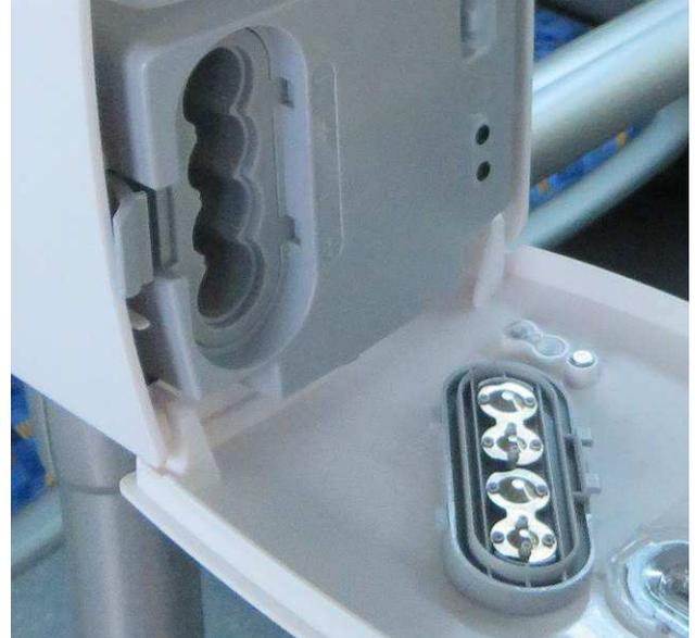
Insert 4 pcs new AA alkaline batteries so that the polarity of the inserted batteries matches the polarity markings on the dispenser control unit body.
