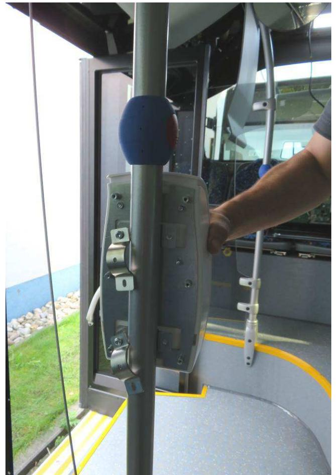
Mount the second screws (8) and tight them evenly to assure the same gaps between the main bracket plate (3) and the brackets (5).
