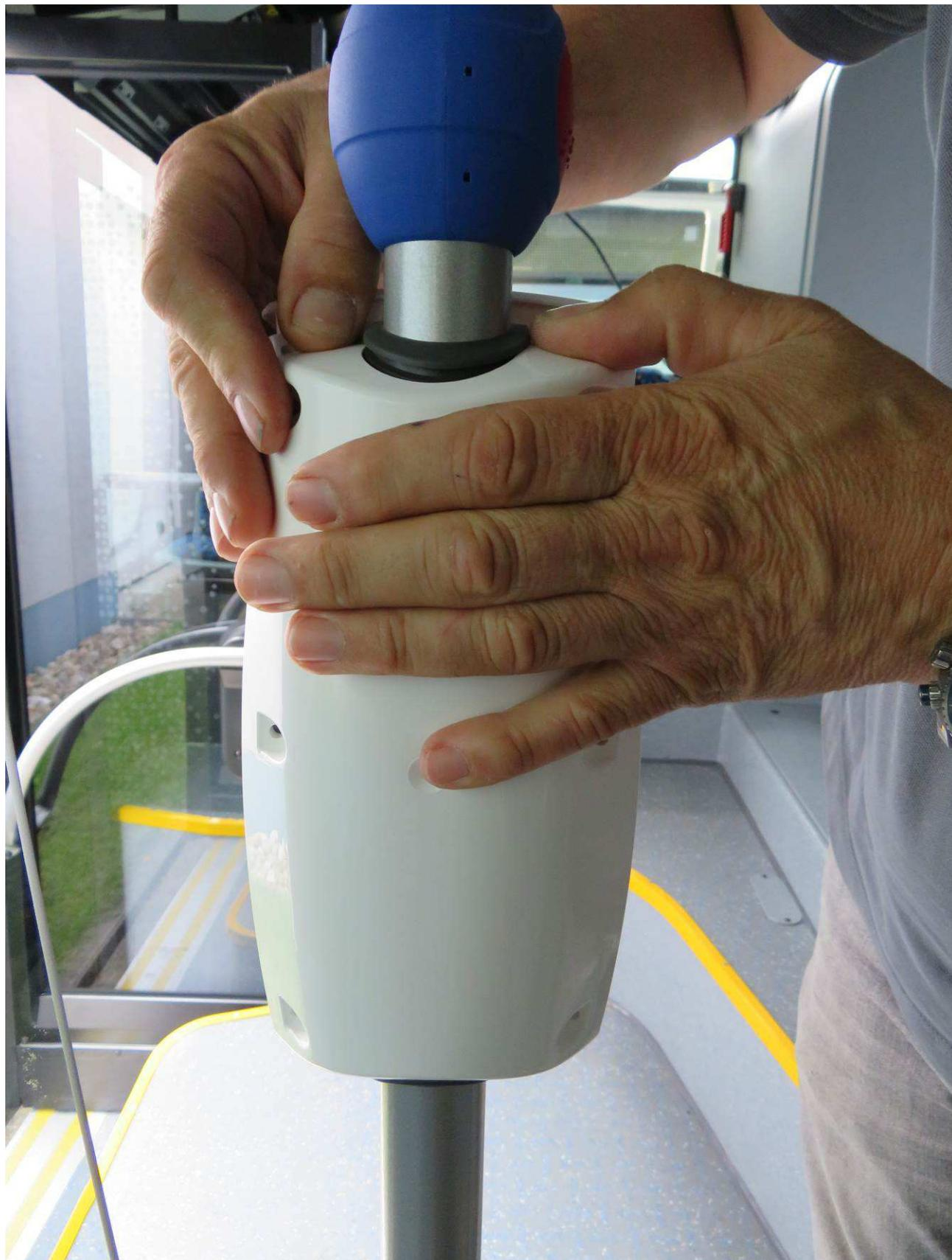
Use 6 screws ⑪ to firmly attach the back cover to the dispenser body.
