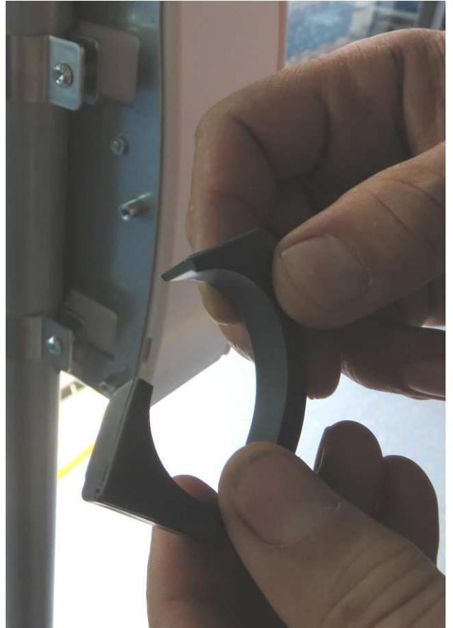
Place the gaskets (7) on the pole (2 pcs) on the upper and bottom side of the dispenser so that the gaskets fit exactly into the slots in the metal holder of the dispenser (3).
