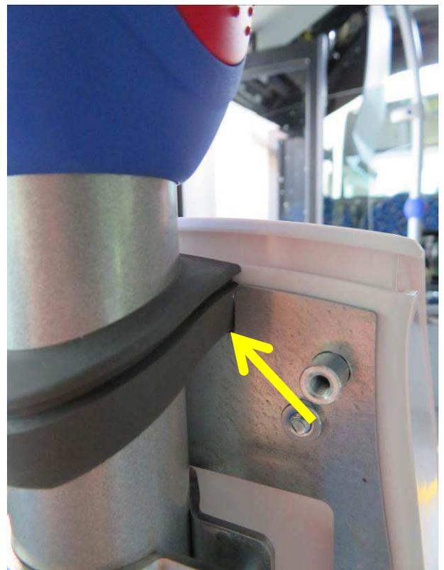
Place the rear cover of the dispenser (6) - first the lower side and then the upper side and check that the rear cover fits exactly into the grooves of the gaskets.
